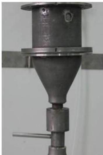
**Fig.1 Self-designed porous media combustor**
