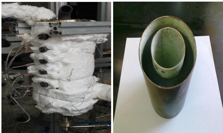
**Fig.4 Self-designed reformer (left) and the Ni-based monolith catalyst (right)**
