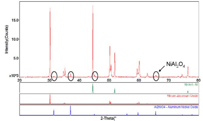
Fig. 4. XRD patterns of sintered anode support material (Ni–YSZ)<sub>0.95</sub>(Al<sub>2</sub>O<sub>3</sub>)<sub>0.05</sub>.
