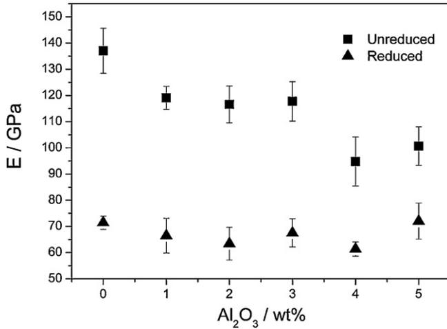
Fig. 3. Young's modulus of as-sintered NiO–YSZ–Al<sub>2</sub>O<sub>3</sub> or Ni–YSZ–Al<sub>2</sub>O<sub>3</sub> composites as a function of alumina content.
