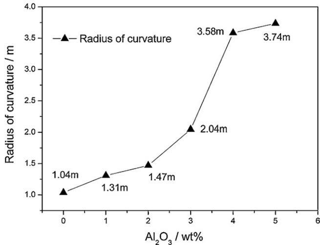
Fig. 1. Radius of curvature as a function of alumina content before H<sub>2</sub> reduction.
