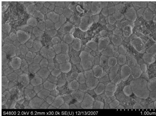
Fig.6 FESEM micrographs of surface of 20 wt% NiO-YSZ anode support before reduction
