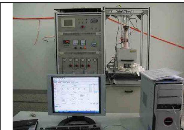
Figure 8 A set-up of cell testing for planar SOFCs
