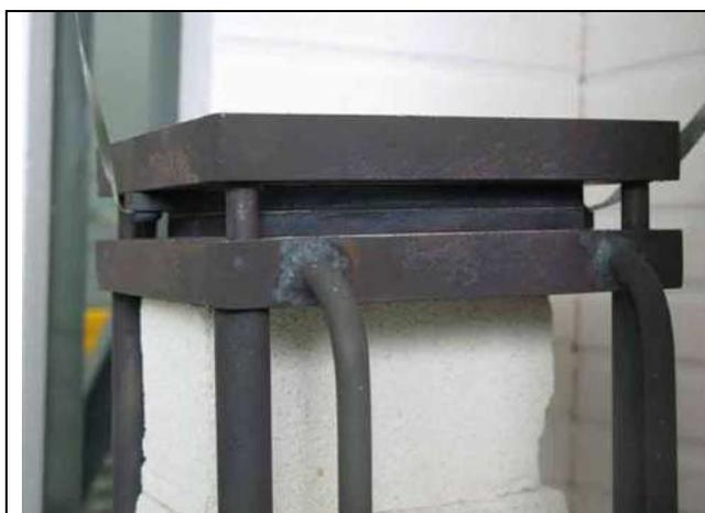
Figure 10 A three cell short stack after testing.
