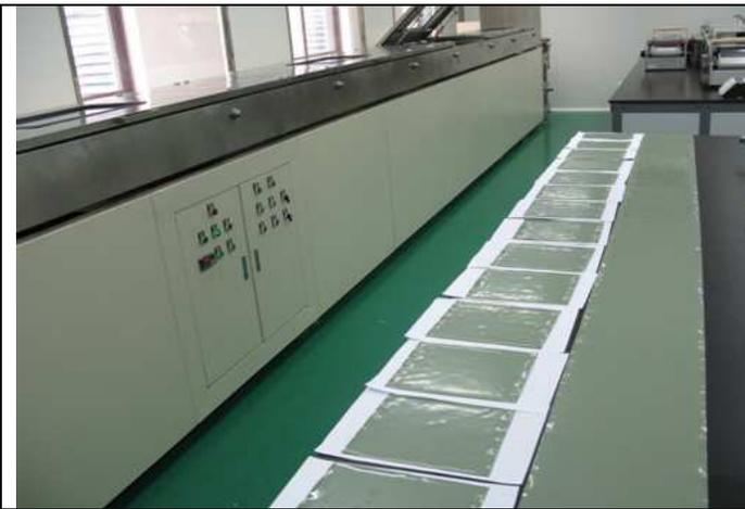
Figure 6 Tape casting machine and anode support green tapes.
