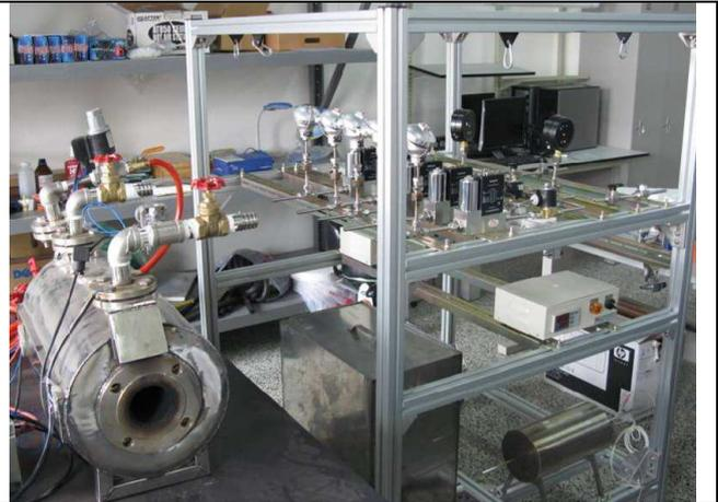
Figure 13 A fuel cell testing system with all the functions to be examined.
